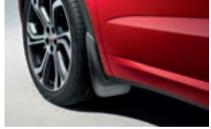
Splash Guards - Front and Rear Jaguar branded front and rear splash guards complement the lines of your vehicle, reduce spray and provide protection from dirt and stone chippings.
