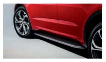
**Fixed Side Steps**The side steps aid entry and exit to the vehicle and improve access to the roof.
